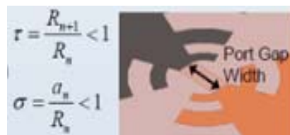
Fig.2. Port Gap Width of Planar Toothed Log Periodic Antenna
